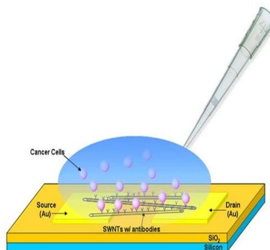
Figure 2. Y-shaped antibodies attached to the nanaotubes,targetting the spherical shaped tumor cells.
