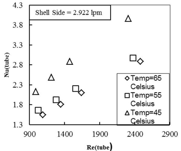
Fig: Nusselt Number vs Process side Reynold's number for a fixed shell side flow-rate
