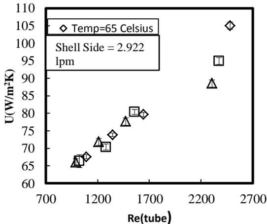
Fig: Overall Heat transfer coefficient vs Process side Reynold's number for a fixed shell side flow-rate
